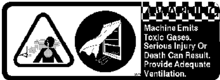
EMISSIONS LABEL - Located Below The Operator's Seat.
